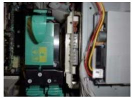
**e.** Remove five screws and pull out the disk cage gently away from the server chassis.
